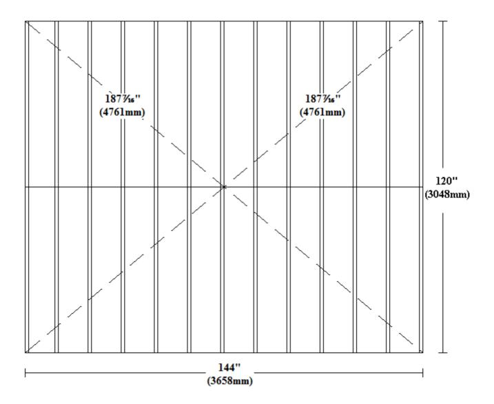
NB:- Floor joists run from gable to gable.
